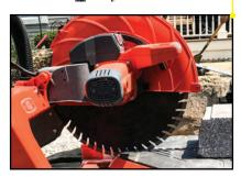
**iQ POWER MANAGEMENT** Soft-start technology controls the input power ramp up for a smooth, uninterrupted operation.
