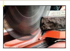
VACUUM SYSTEM Dust is captured within the blade guard, rear dust guard, and downdraft louvered table via a high-powered, integrated vacuum system
